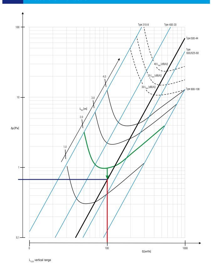
Instruction: Attention, diagrams refer to diffusers with horizontal blades. For oblique blades it is recommended to use an appropriate selection chart. Air stream range  $Q_h$ =100  $m_{\text{s}}/h$  and vertical range  $L_{\nu_0,25} < 2m$ . Sought after diffuser size. We draw a horizontal line (red) corresponding to  $Q_h$ =100  $m_{\text{s}}/h$  until curve
